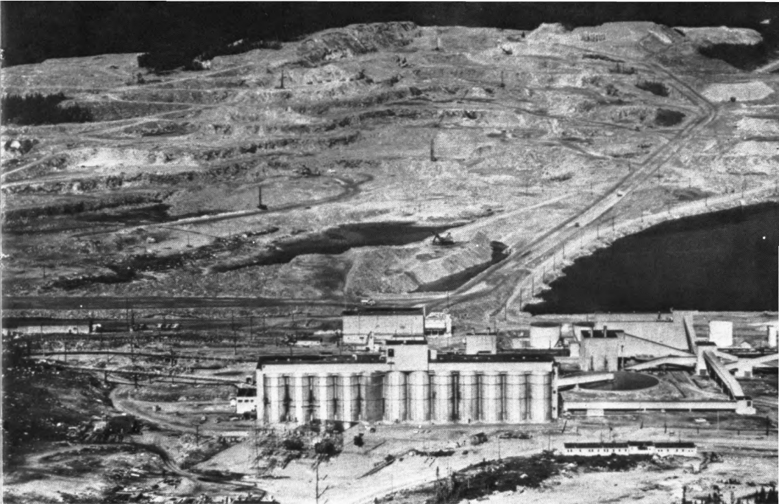
69 An aerial view of Lac Jeannine mine, part of the Quebec-Cartier iron ore project in Canada. Production rate is about 20 million tons per year, and the picture shows the 40 foot terraces from which the ore is stripped
